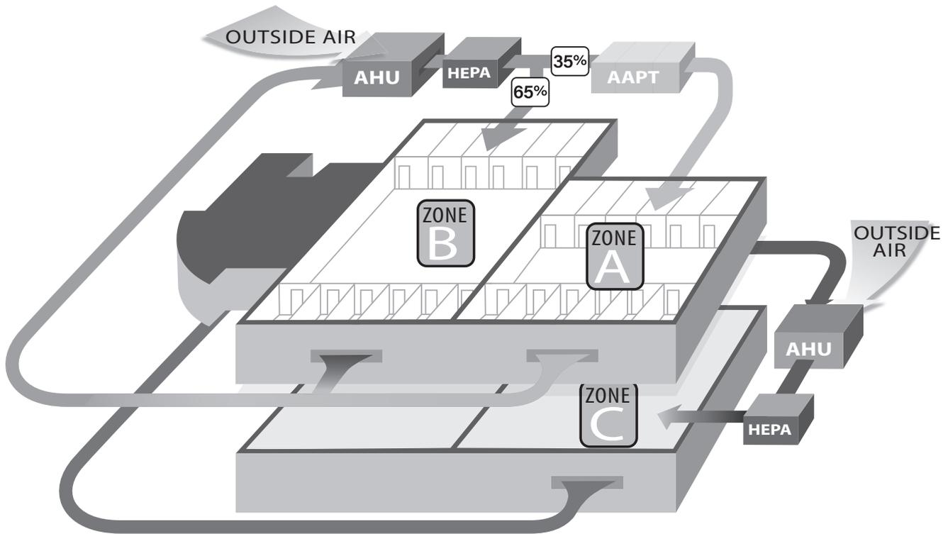
Fig. 1. Schematic representing zones A, B, and C and the existing heating ventilation and air conditioning layout for all zones.
